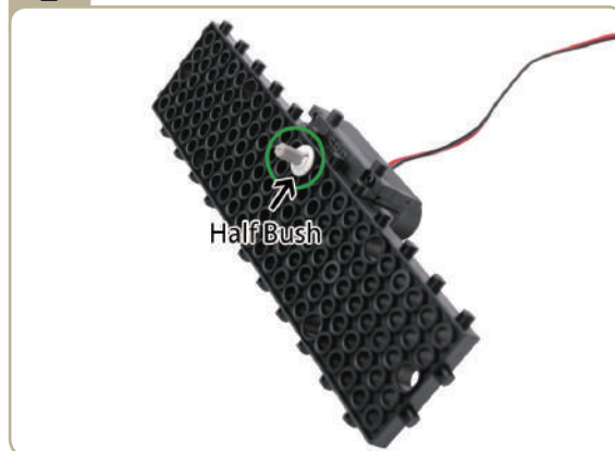
Insert a half bush to the shaft of DC motor.
